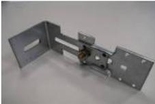
Adjustable bracket for anchoring the vertical wooden support batten of to structures with uneven back (e.g. uneven masonry walls) and to create an insulation and ventilation cavity (60 to 120 mm to the back of the batten).
