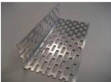
0.8 mm thick perforated aluminum profile used to seal the 50 mm cavity in the façade to prevent birds and pests from entering. The raised leg of the sealing profile is clamped between the wooden support batten and Bluclad Proboard.
