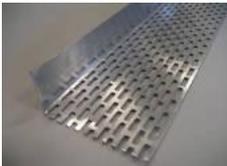
0.8 mm thick perforated aluminum profile used to seal the 70 mm cavity in the façade to prevent birds and pests from entering. The raised leg of the sealing profile is clamped between the wooden support batten and Bluclad Proboard.
