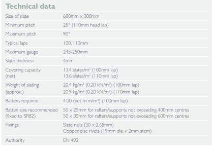
Cedral Supercem slates are manufactured to EN492, Type NT, 4.0mm thick Fibre Cement Slates in Ireland, with a nominal average density of 1970 kg/m³ and a minimum apparent density of 1750 kg/m³. They have a smooth surface with a square edge and are offered with a 10 year manufacturer's colour guarantee and a 30 year structural guarantee.
