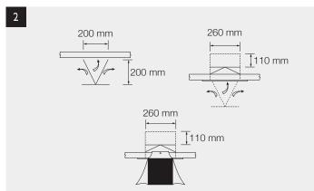
Cut underlay in a "V" shape as shown. Fold back cut edges of underlay.
