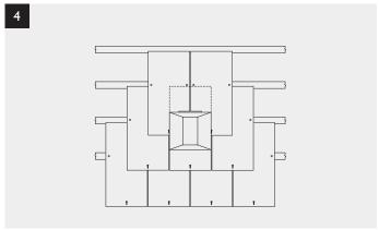
Position the vent slate. Drill two 4.5mm holes in the vent slate, centred on the slating batten and fix to batten through the nail holes provided.
