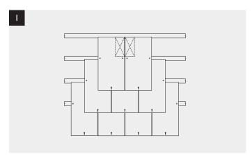
Complete the slating in the normal manner to one course below the required position for the slate vent.
