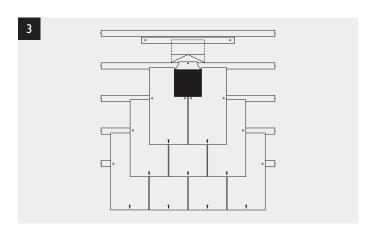
Cut the two slates, which will be under the vent slate to give the required clear air space. The amount to be cut from these slates will vary according to the size of the slate, the lap and gauge of the slating.
