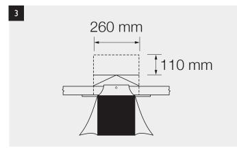
Secure the felt weir by folding the top section of cut underlay over the batten and fix in place with a 20mm galvanised clout nail to the face or back edge of the batten.
