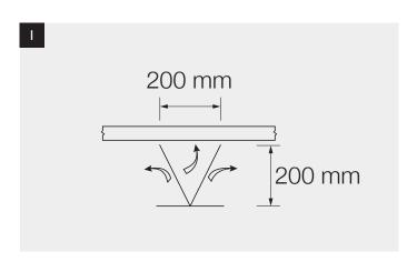
Cut underlay in a 'V' shape as shown. Fold back cut edges of underlay. Using the Cedral Felt Weir will give additional protection to the underlay cut.
