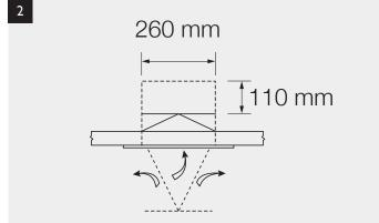
Neatly cut a 260mm long slot in underlay, at a distance of approx. 60mm above top of the slating batten. Slide the felt weir through this slot until the upstand of the felt weir is up to the bottom of the batten. Allow a minimum cover of 110mm between the felt weir and the underlay.
